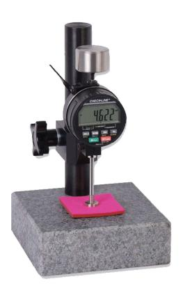
Accurately measures thickness of textiles, non-wovens, technical fabrics and many other materials. Using specific diameter presser foot (feeler) and mass (weight) it can measure according to ASTM D1777, ISO 5084, D1621, D5199, D461, D751-06, D3652, ISO 9863-1, ISO 964-1 (2 kPa only) and many other international testing standards.
