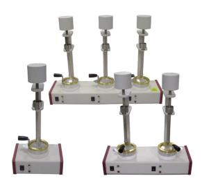
To determine the oil or finish content of wool or synthetic samples by solvent percolation and evaporation. Suitable for fiber, yarn or fabric. Available with 1, 2 or 3 extraction units. To be fully compliant with Edana method ERT 155, it needs a large extraction tube- 12 mm (OD), 10 mm (ID). (Full title of new method is: DETERMINATION OF ACETONE EXTRACTABLE FINISH ON NONWOVENS).
